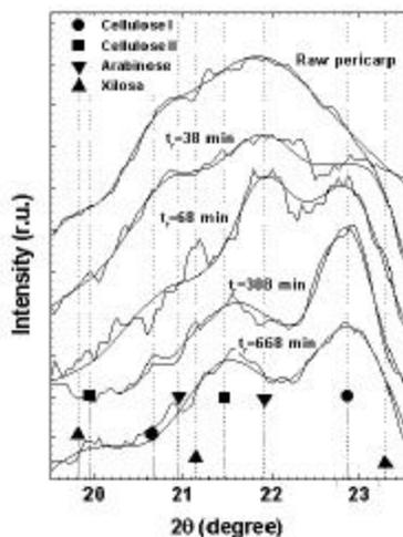
Fig. 2 X-ray diffractograms for pericarp taken at different *nixtamalization* times
