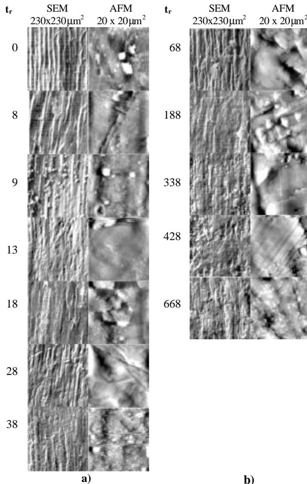
Fig. 11 Morphological evolution of the corn pericarp through a) cooking stage and b) steeping stage in the same *nixtamalization* process. 230 x 230 μm<sup>2</sup>: SEM images, 20 x 20 μm<sup>2</sup>: AFM images;  $t_r$  in minutes.
