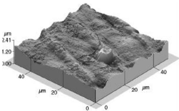
Fig. 9 3-D AFM 50 x 50 μm<sup>2</sup> image showing the fibrillar structure of the raw corn pericarp.
