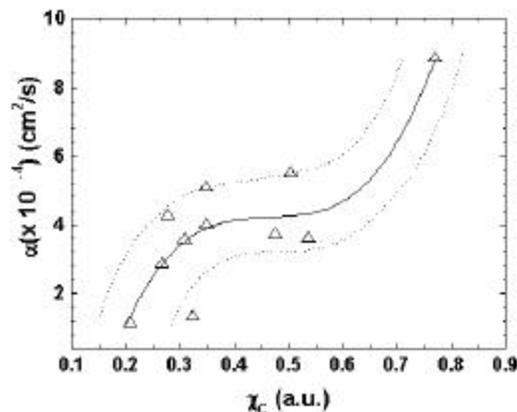
Fig. 7 The relationship between the thermal diffusivity and crystallinity of the nixtamalized corn pericarp.
