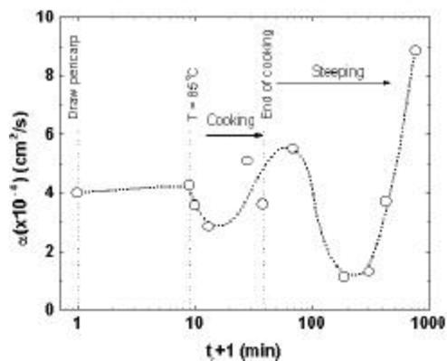
Fig. 6 Thermal diffusivity of the corn pericarp at different nixtamalization times.
