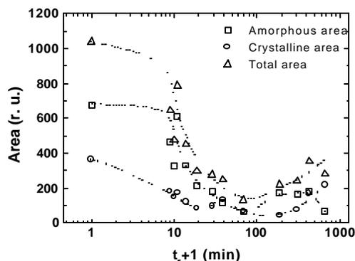
Fig. 4 Behavior of the amorphous, crystalline, and total areas of the x-ray diffractograms as function of the *nixtamalization* time.
