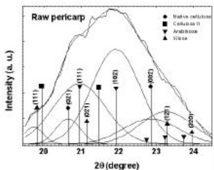
Fig. 1 Deconvoluted x-ray diffractogram of raw corn pericarp.
