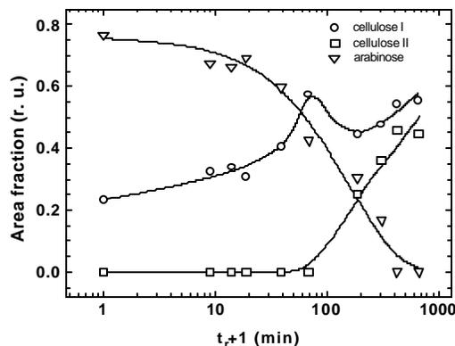
Fig. 3 Area fractions of the normalized native-cellulose, cellulose-II and arabinose peaks as function of *nixtamalization* time.
