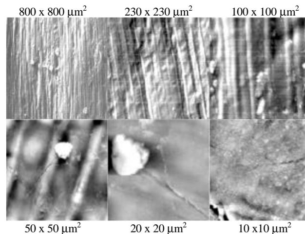
Fig. 8 SEM (a) and AFM (b) images of raw corn pericarp at different magnifications (upper images are SEM and lower AFM)
