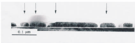
Figure 13. Bright field XTEM micrograph of a Fig. 12 sample. The GaN and Si are viewed in the [11\bar{2}0] and [1\bar{1}0] projections, respectively. Multi-beam conditions.
